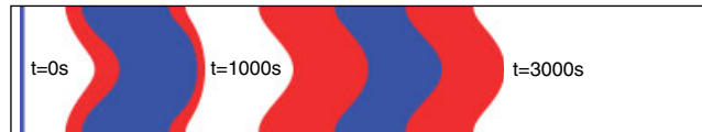
Figure 12. Shear dispersion: contours at t=0 s, 1000s and 3000s (the line source at t=0 s is exaggerated for clarity in the above figure).
